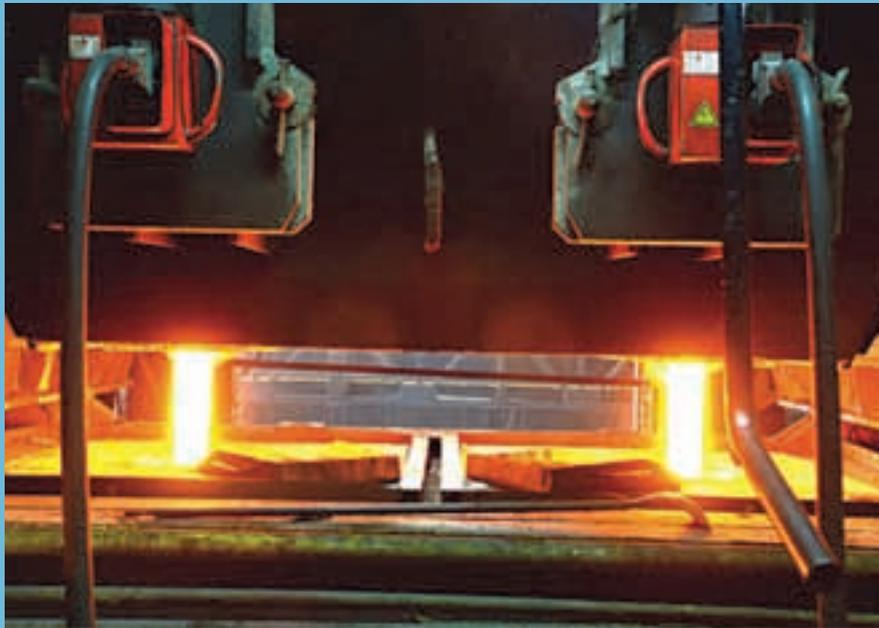
*Concast Machine at Steel Melting Shop.*
